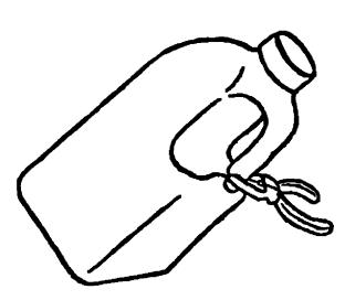
2 Remove the candle and quickly 'pinch' the soft base of the handle with pliers so that the base is sealed tight to prevent water flowing through it. Hold the pliers there until the plastic cools, ensuring that the seal is completely closed.
