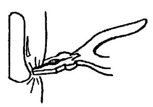
3. When the base is soft, pinch the base closed with a pair of pliers and then let it cool. Make sure that no water can flow through the pinch-closed base.
