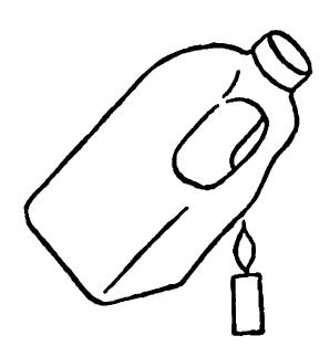
Take a plastic container with a hollow handle. Gently warm the base of the handle over a candle, turning the handle around until the base of the handle is shiny and soft all the way around.
