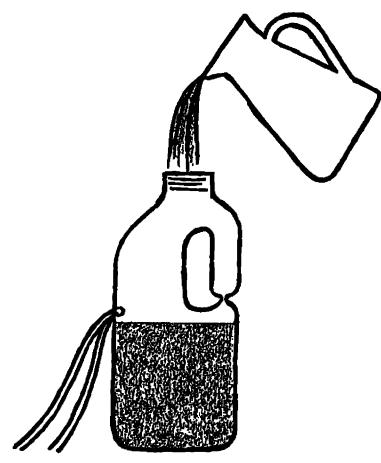
Pour water into the tippy tap until the water is almost level with the holes in the back of the bottle. Use the stick to hang the tippy tap in the bathroom or outside in a tree. The tippy tap is now ready for use.
